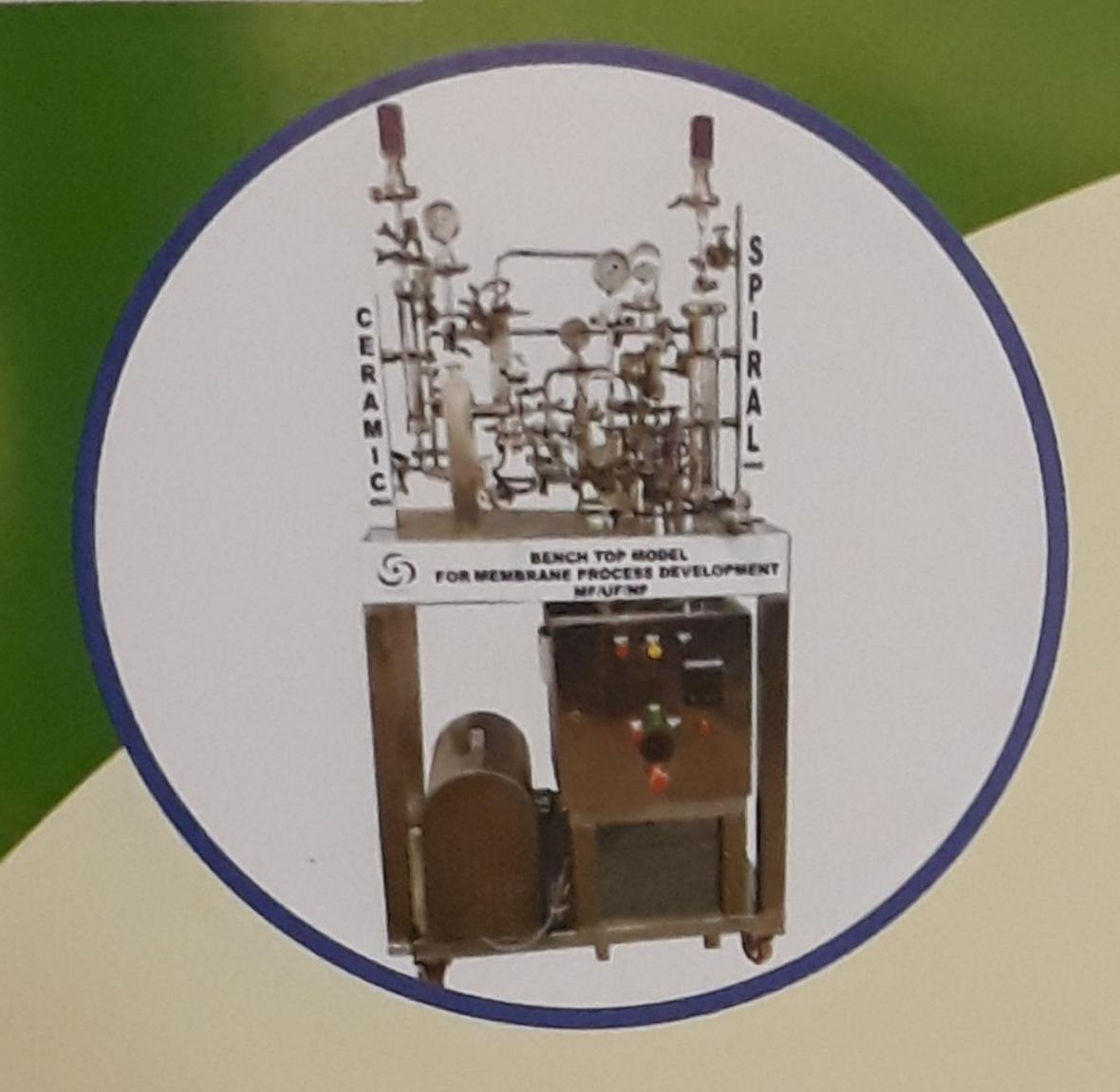
User friendly bench top laboratory membrane device for various unit operations like microfiltration, Ultrafiltration, nanofiltration and reverse osmosis.
